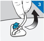
Detach tube from groove in fixation plate
